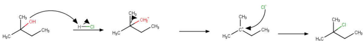
Figure 1: S_N1 2-methyl-2-butanol to 2-chloro-2-methylbutane Mechanism
